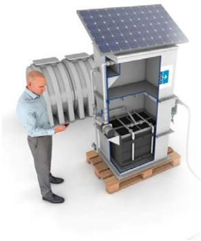
AQUA CUBE is a cost effective, compact and mobile water treatment plant based on a modular membrane filtration system that enables available water resources to be used in particular purposes such as service water or drinkable water. AQUA CUBE is easy to install and operate, has a very low energy consumption, and it is ready to use. AQUA CUBE is able to remove up to 99.99999% of bacteria and other pathogens out of polluted water by means of ultrafiltration filters, and make it drinkable.
