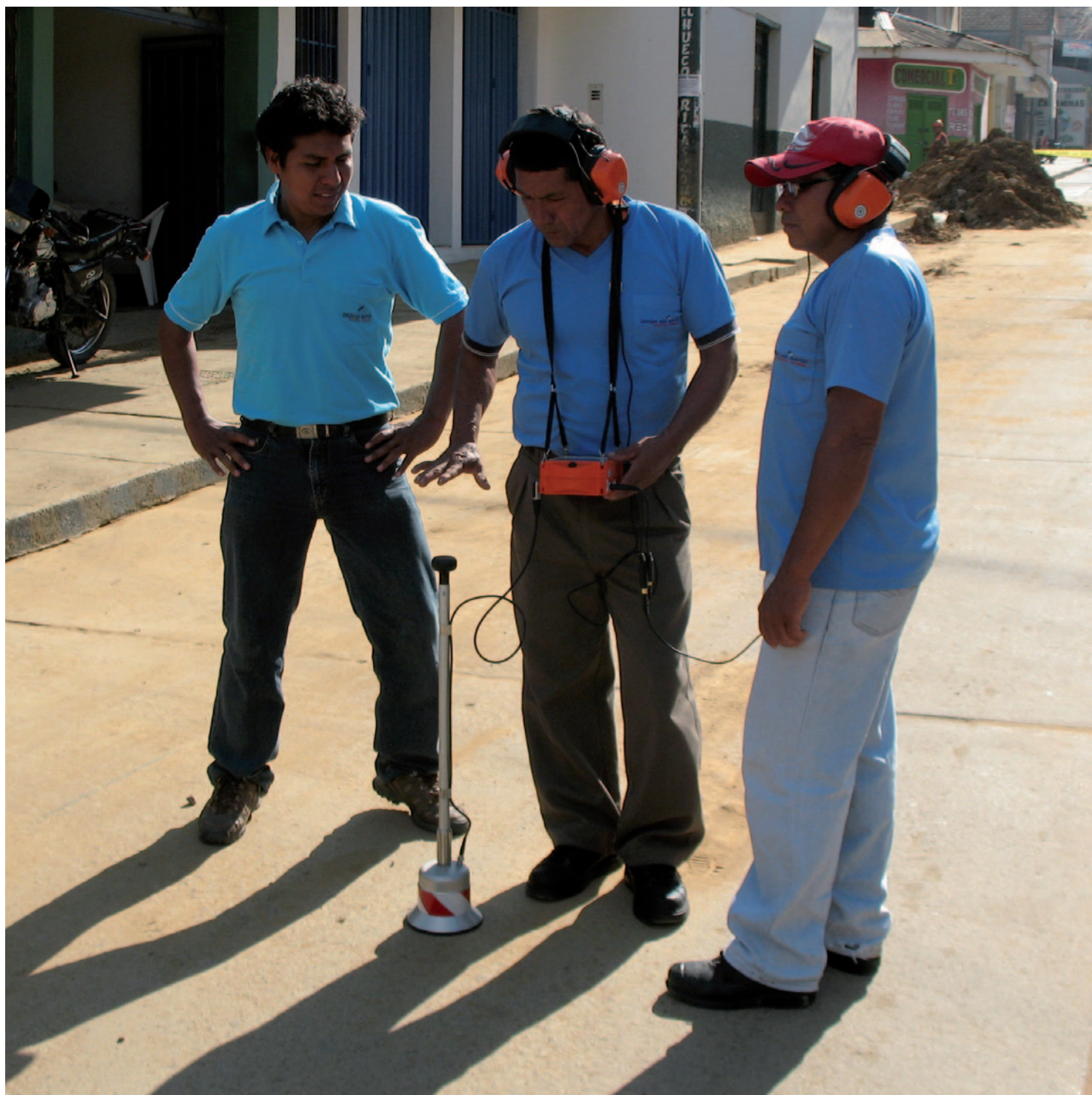
Figure 20: Water leak detection (Hermann Sewerin GmbH)
